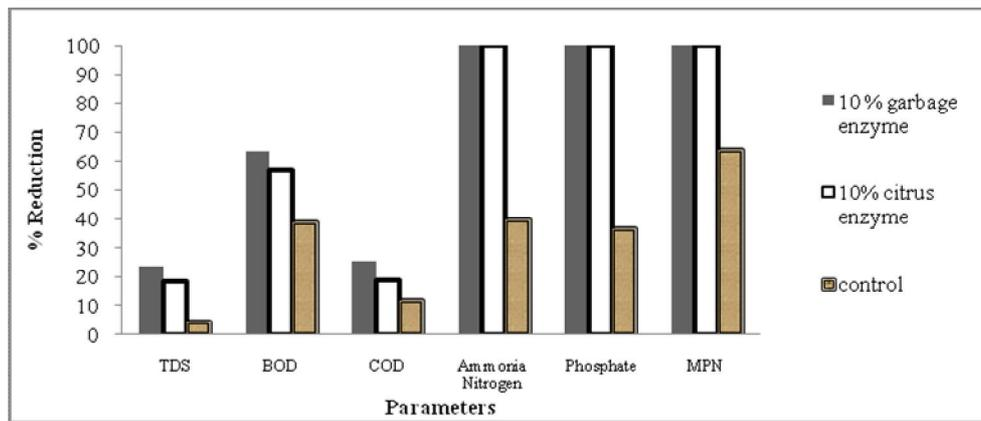
Fig. 2. Percentage reduction of various parameters after treatment of synthetic greywater with 10% garbage & 10% citrus enzyme solution after 5 days.
