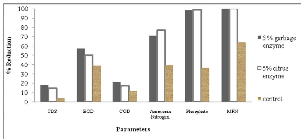
Fig. 1. Percentage Reduction of various parameters after treatment of synthetic greywater with 5% garbage & 5% citrus enzyme solution after 5 days.
